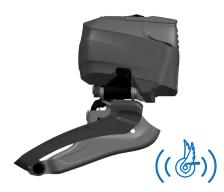
The front derailleur LED flashes in high frequency to indicate the failed coupling.
