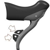
**2)** Hold down the right and left Ergopower control MODE buttons at the same time for approx. 5 seconds until the PINK led turns on.
