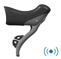
The LED remains flashing in high frequency **until the control is coupled to the rear derailleur**: if after **90 s** it continues to flash, and therefore it is not coupled, the LED turns off.
